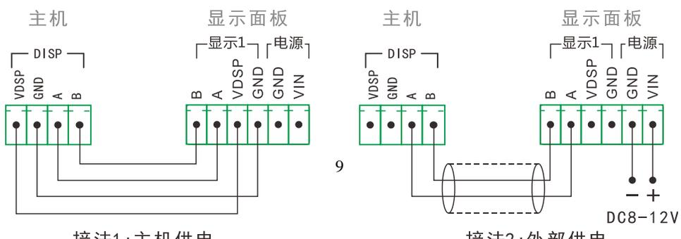
Fig. 4.11 Connection Method between Host and Display Panel
