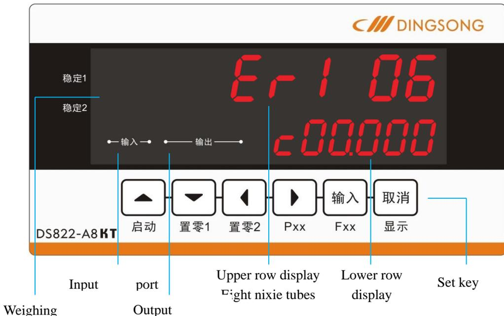
Figure 3.3 function diagram of display panel (front)
