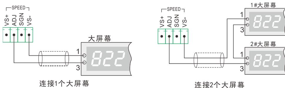
Figure 4.7 Schematic diagram of connection of large screen display
