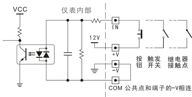
Figure 4.1 schematic diagram of switch input connection
