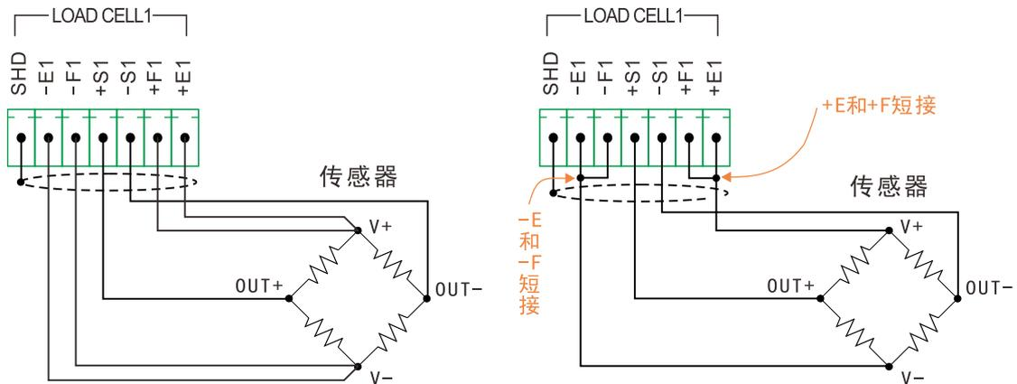
Figure 4.8 6-wire connection method of load cell Figure 4.9 4-wire connection
