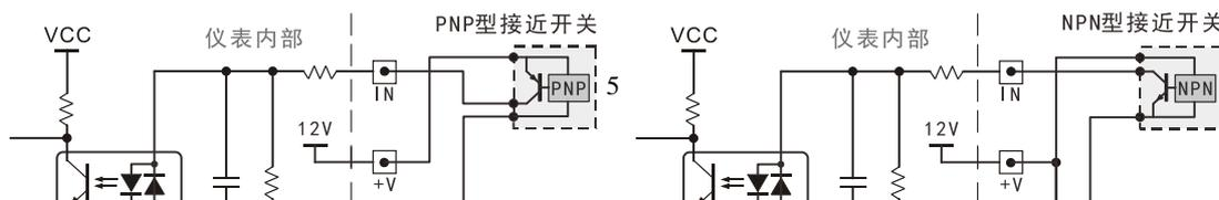
Figure 4.2 Schematic diagram of PNP proximity switch connection Figure 4.3 Schematic diagram of NPN proximity switch connection
