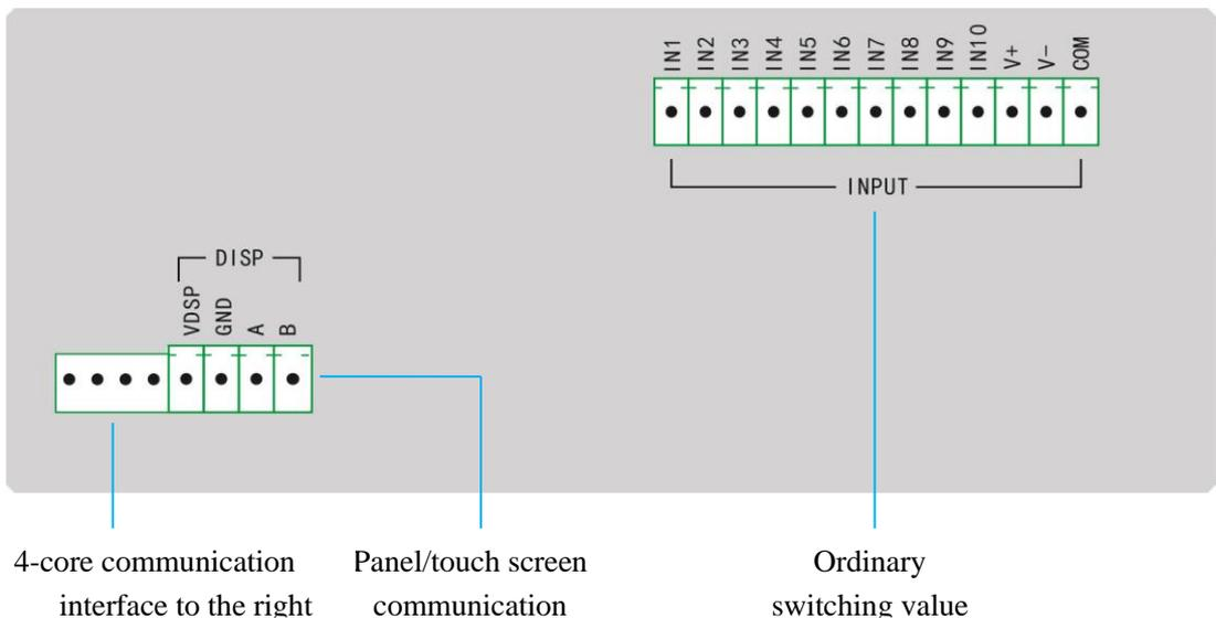
Fig. 3.1 function diagram of a side of host panel
