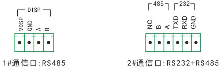
Figure 4.10 Schematic diagram of two communication interfaces of the instrument
