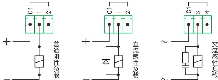
Figure 4.5 Schematic diagram of relay output connection
