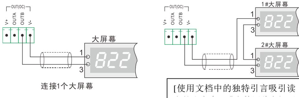
Figure 4.7 Schematic diagram of connection of large screen display
