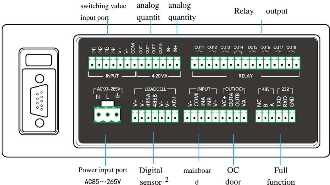
Figure 3.2 Functional Schematic Diagram of B Side of Host Panel
