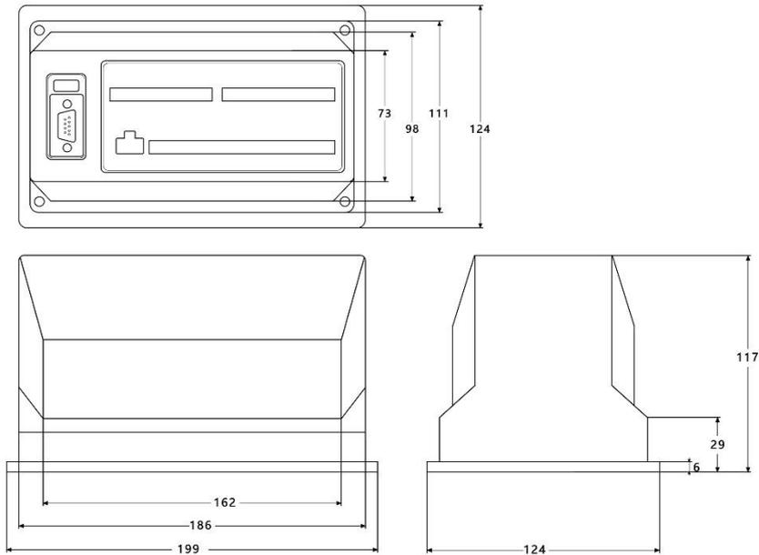
Figure 2.1 Installation Dimensions of Host
