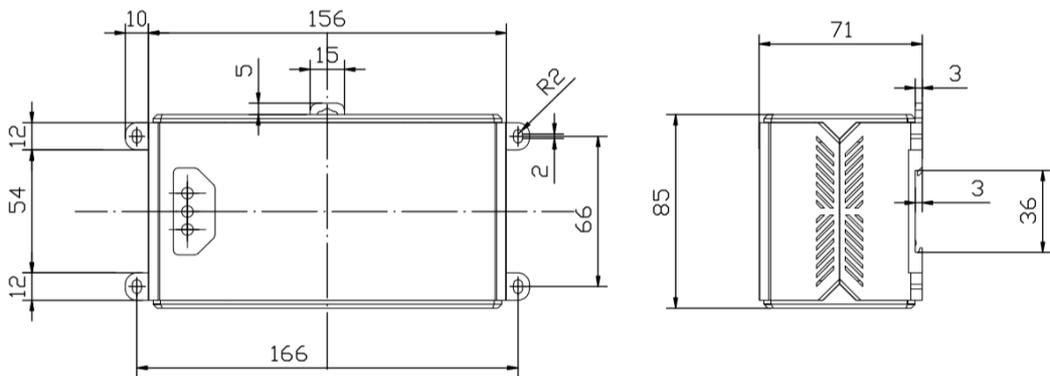
Figure 2.1 Installation Dimensions of Host
