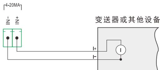
Figure 4.10 Schematic diagram of 4-20mA analog input connection
