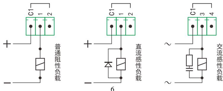
Figure 4.5 Schematic diagram of relay output connection
