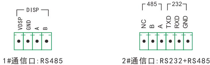
Figure 4.14 Schematic diagram of two communication interfaces of the instrument
