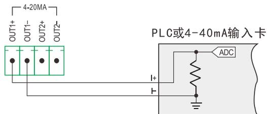
Figure 4.9 Schematic diagram of 4-20mA analog output connection
