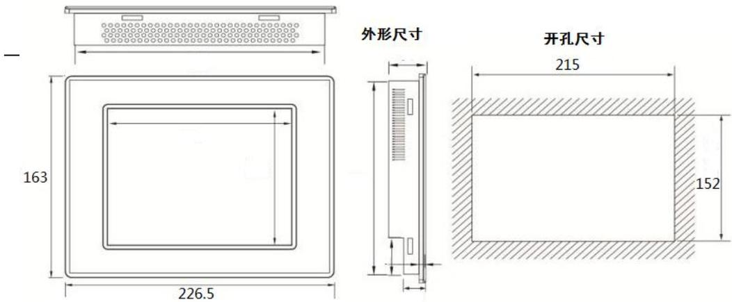
Figure 2.3 Installation Dimensions of Touch Screen
