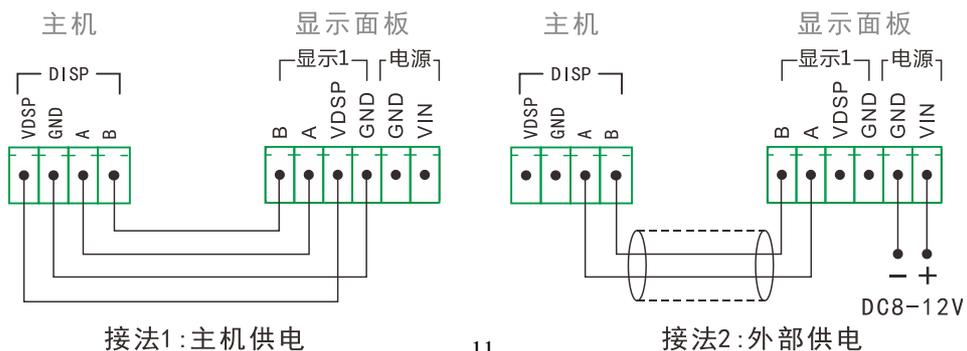
Fig. 4.15 Connection Method between Host and Display Panel
