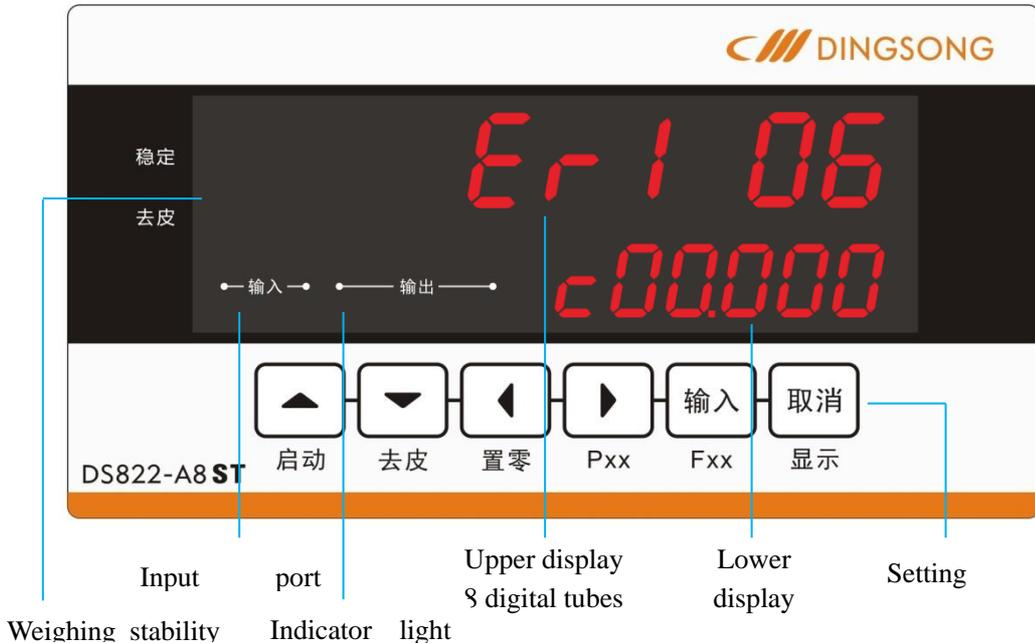
Figure 3.3 Functional diagram of display panel (front)
